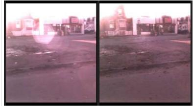
Glare removal: the image on the left was taken with a standard camera. The image on the right comes from a camera modified with a pinhole mask. The photograph is then treated with software to generate a glare-free image. Credit: Amit Agrawal, MERL
