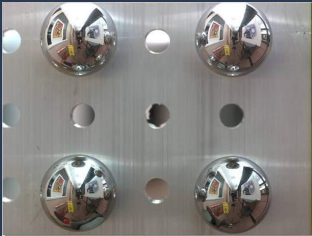
Camera looking into four spherical mirrors
