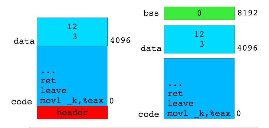
Image file has header (tells loader what to do) Memory image has bss segment!
