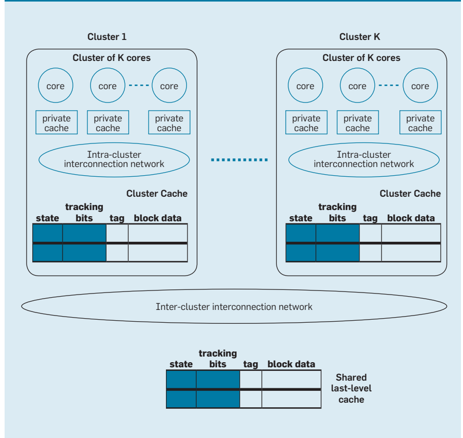
Figure 2. Hierarchical system model; additions for coherence are shaded.
