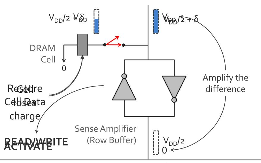
In the stable state, sense amplifier drives the cell
