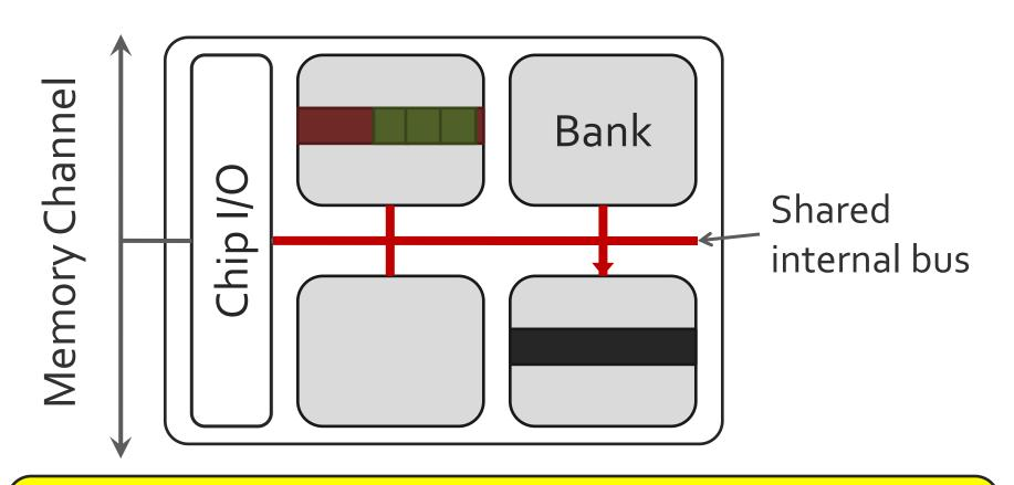
Overlap the latency of the read and the write 1.9X latency reduction, 3.2X energy reduction
