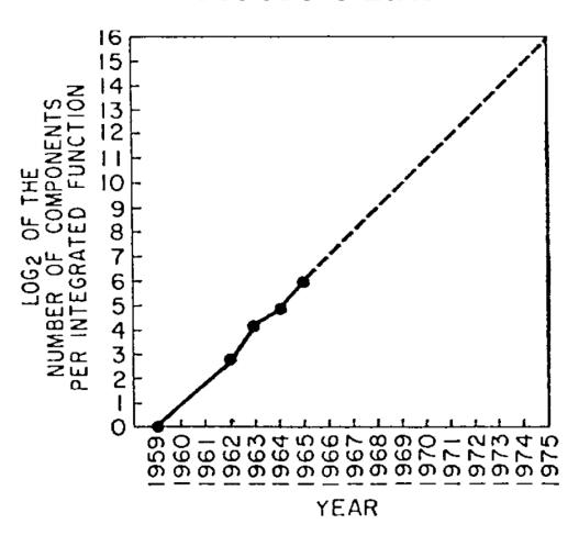
Number of components [transistors] per integrated function [integrated circuit] will double every year (for at least ten years).
