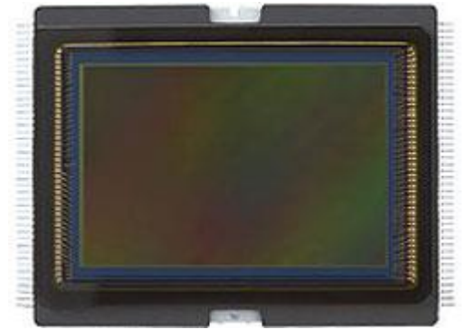
Canon 6D sensor (20.20 MP, full-frame)
