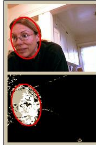
Figure 3. The normal and face-probability views as Camshift tracks my face. In the face-probability view, black pixels have the lowest value, and white, the highest. Gray pixels lie somewhere in the middle.
