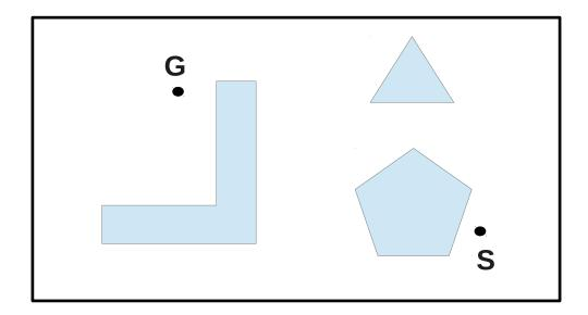
b) Draw the visibility graph (4 pts). Highlight the shortest path between S and G using the L2 metric (1 pt). Why is this the shortest path (2 pts)?
