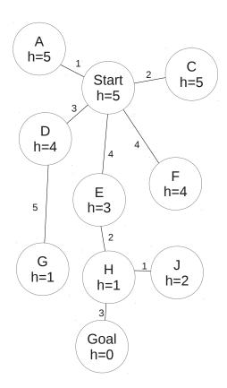
The order that you remove the edges can have a significant impact on the length of the resulting path. For this question you will first develop an algorithm to generate a tree from a cyclic graph using a breadth first search starting with the *Start* node as the root. Next you will do the same but use a depth first search. Both algorithms should be written concisely in pseudocode (use the back as necessary) (4 pts each).
