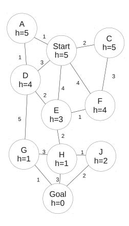
b) A spanning tree is a method for reducing a cyclic graph to a tree. One way to construct a spanning tree is to simply remove edges until there are no more cycles but the graph remains connected. An example spanning tree for the above graph is:
