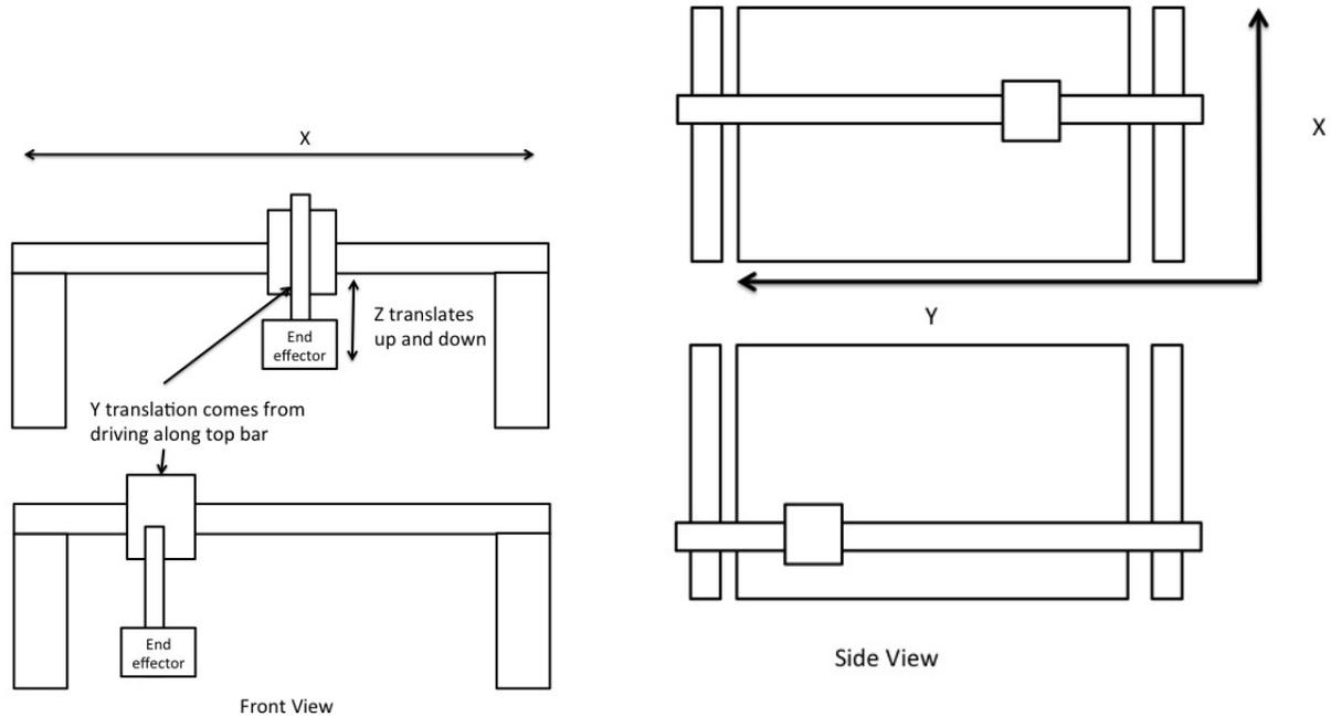
This robot has 3 linear actuators: one actuator moves in  $x$ , one moves in  $y$  and one moves in  $z$  with an end effector attached to the the end of the  $z$  actuator.
