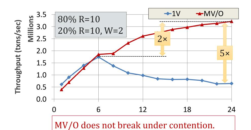
MV/O does not need throttling for max perf.
