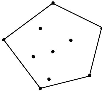
This figure shows the convex hull of 10 points.
