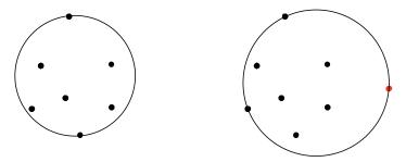
In the example on the left, only two points are on the smallest enclosing circle. On the right we've added a new point (colored red) to the set. The new point was outside of the previous smallest enclosing circle. The new solution has three points on the circle, including the new red point.
