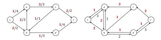
Finally, there is one more augmenting path,  $s \rightarrow a \rightarrow b \rightarrow d \rightarrow t$  of capacity 2. This gives us the maximum flow that we saw earlier (left). At this point there is no longer a path from *s* to *t* in the residual graph (right) so we know we are done.
