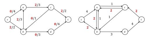
If we continue running Ford-Fulkerson, we might find the *augmenting path*  $s \rightarrow a \rightarrow c \rightarrow b \rightarrow d \rightarrow t$  which has capacity 1, bringing the flow value to 3, and yielding the following flow (left) and residual graph (right).
