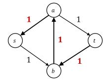
Unlike before, there is now an *s*-*t* path with capacity 1! The path  $s \rightarrow b \rightarrow a \rightarrow t$  "undoes" the flow that was originally pushed through  $a \rightarrow b$  and redirects it to  $a \rightarrow t$ , thus improving the flow and making it optimal.
