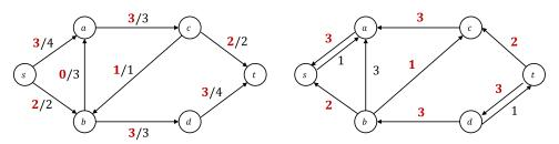
We can think of Ford-Fulkerson as at each step finding a new flow (along the augmenting path) and adding it to the existing flow. The definition of residual capacity ensures that the flow found by Ford-Fulkerson is *legal* (doesn't exceed the capacity constraints in the original graph). We now need to prove that in fact it is *maximum*. We'll worry about the number of iterations it takes and how to improve that later.
