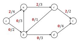
An important observation we have just made is that if we add a constant amount of flow to all of the edges on a path, we never violate the flow conservation condition since we add the same amount of flow in and flow out to each vertex, except for s and t. As long as we do not violate the capacity of any edge, the resulting flow is therefore still a feasible flow.
