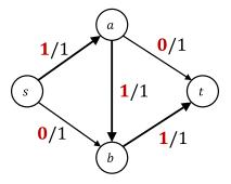
Are there any *s*-*t* paths with available capacity left? No, there are not. But is this flow a maximum flow? Also no, because we could have sent 1 unit of flow from  $s \rightarrow a \rightarrow t$  and 1 unit of flow from  $s \rightarrow b \rightarrow t$  for a value of 2. The problem with this attempted solution was that
