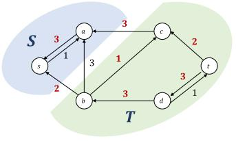
It must be that  $t \in T$  since otherwise *s* would be connected to *t*, so this is a valid *s*-*t* cut. Let  $c = \operatorname{cap}(S, T)$ , the capacity of the cut in the *original* graph. From our earlier discussion, we know that  $|f| = f(S, T) \le c$ . The claim is that we in fact *did* find a flow of value *c* (which therefore implies it is maximum). Consider all of the edges of *G* (the original graph) that cross the cut in either direction. We consider both cases:
