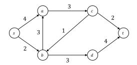
Our goal is to push as much *flow* as possible from *s* to *t* in the graph. The rules are that no edge can have flow exceeding its capacity, and for any vertex except for *s* and *t*, the flow *in* to the vertex must equal the flow *out* from the vertex. That is,
