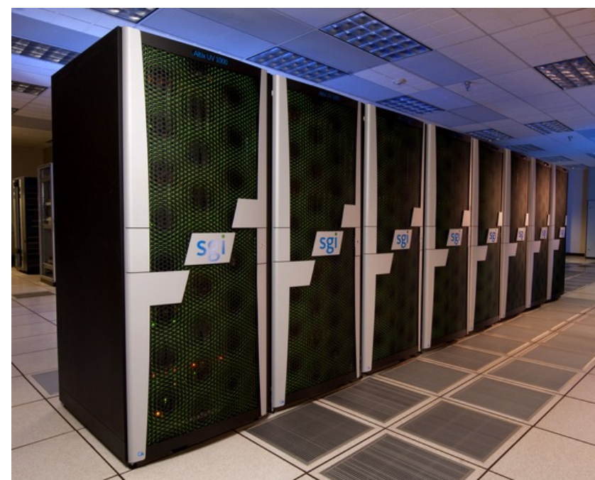
SGI UV 1000cc-NUMA (today) 4096 processor cores
