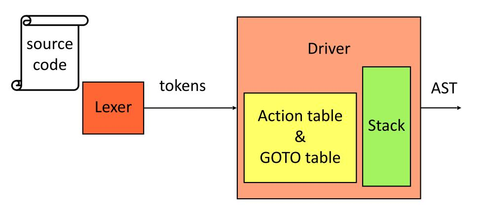
Push down automata: FSM with stack
