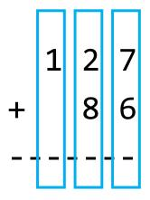
An **n-bit** adder will work the same way, by adding one column of numbers at a time. But it will add **binary** digits, not decimal digits.
