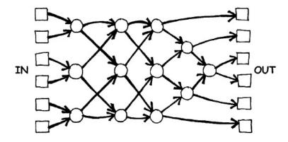
Assume each comparator (i.e. the circles) takes 1 millisecond (1/1000<sup>th</sup> of a second) to compare its two elements and output its results and that the time for a data value to go from one comparator to the next is negligible. We wish to sort 2000 sets of 6 integers each.
