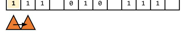
Based on its current state and the value in the cell the device points to, it can change state, change the value in the cell and/or move the device.
