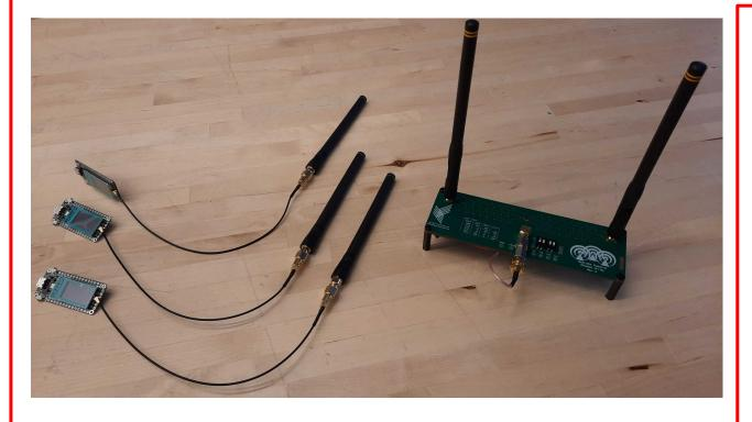
The NulLoRa test node, alongside other 915 MHz devices used as interferers for testing.
