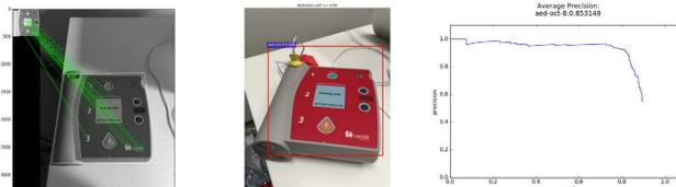
Figure 5. Object Detection Example (left: SIFT, mid: TPOD, right: roc curve for TPOD)
