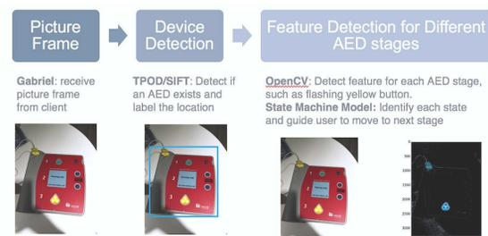
Figure 3. Server Process Pipeline
