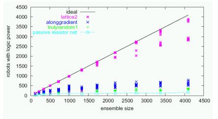
Fig. 11. Robots energized (logic power) for three representative algorithms vs. ensemble size
