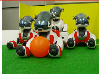
CMTrio, CMPack, CMDash AIBOs, 4-legged, fully autonomous
