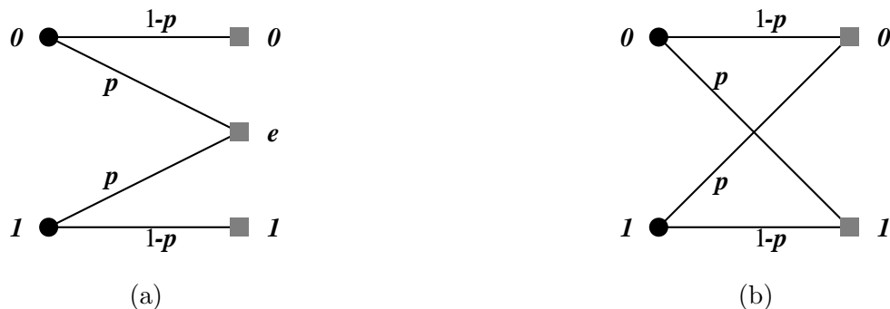
Figure 1: Two examples of channels: (a) The Binary Erasure Channel (BEC) with erasure probability p , and (b) The Binary Symmetric Channel (BSC) with error probability p
