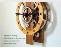
Right side, showing hour divisions on this time ring, weight and pendulum turned from wood.
