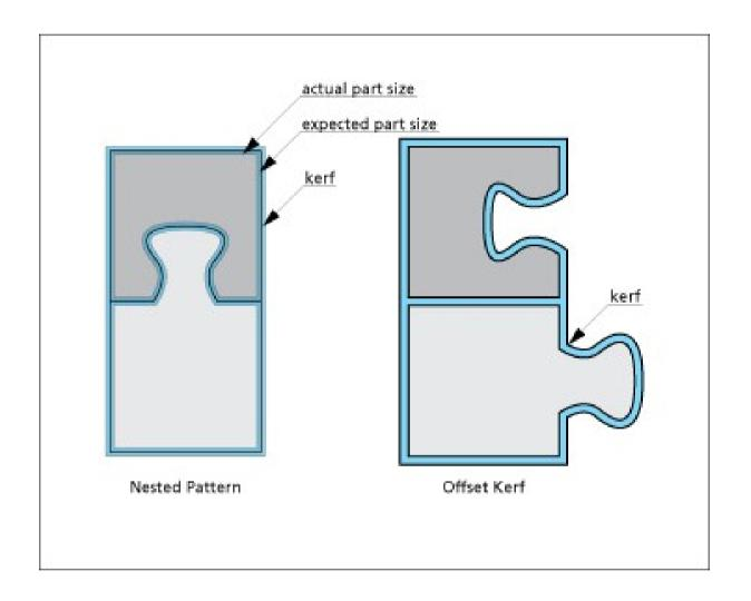
Can do this in SolidWorks with Insert > Faces > Move.
