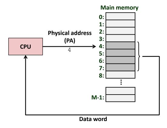
Used in "simple" systems like embedded microcontrollers in devices like cars, elevators, and digital picture frames
