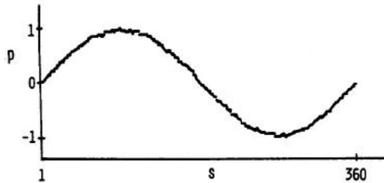
Fig. 6 After sixteen data points are stored. Maximum error = 0.09 and r.m.s. error = 0.033.
