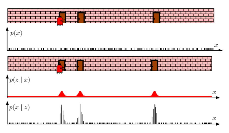
Image from Burgard et al., "Introduction to Mobile Robotics", 2014, lecture 12: "Bayes Filter – Particle Filter and Monte Carlo Localization".
