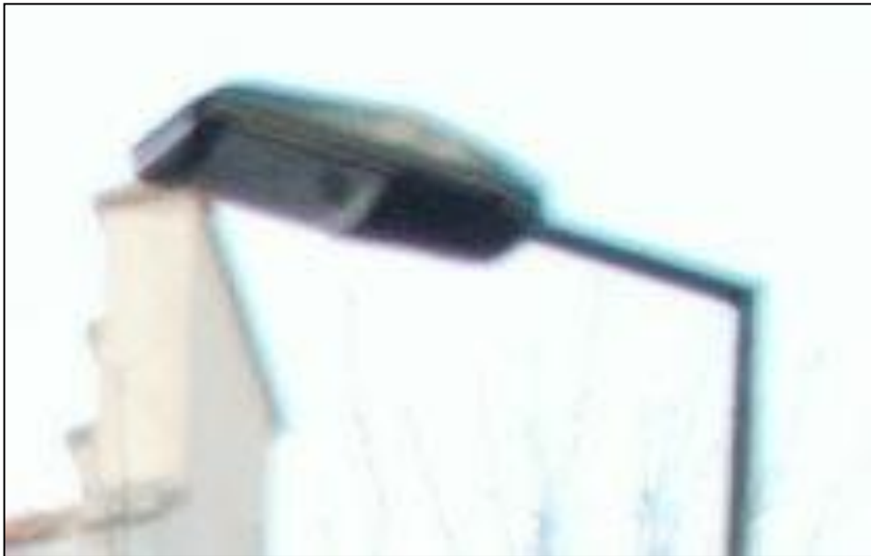
longitudinal chromatic aberration (axial)
