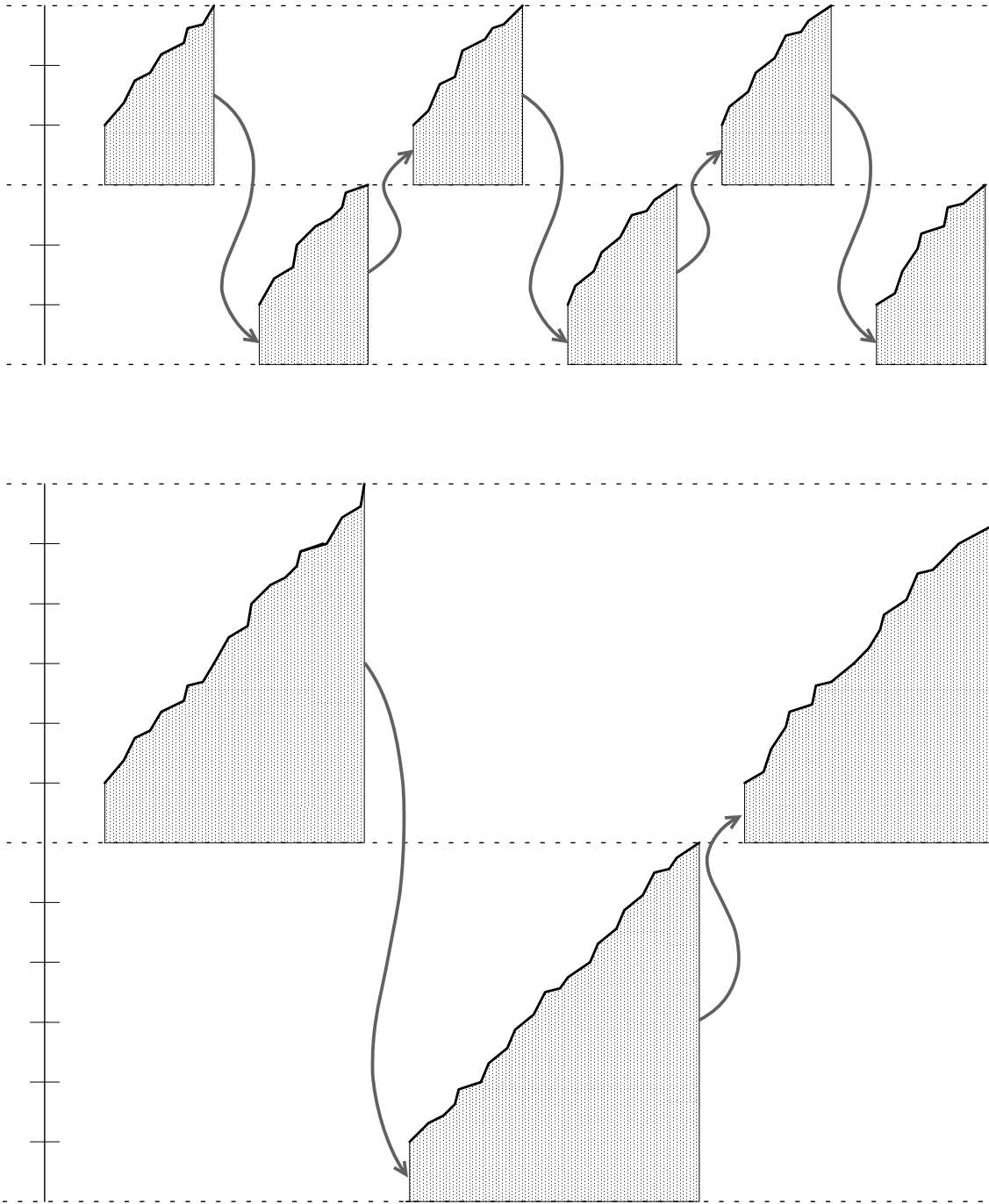
Figure 6: Memory usage in a semispace GC, with 3 MB (top) and 6 MB (bottom) semispaces
