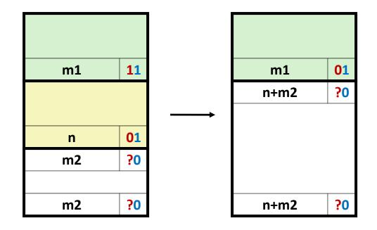
**Header: Use 2 bits (always zero due to alignment):**
