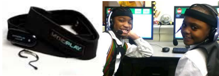
Fig. 1. On the left, NeuroSky's BrainBand. On the right, two students wear BrainBands that log their EEG data while they use the Reading Tutor.
