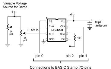
Pinout and connection details for the LTC1298.
