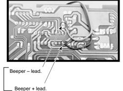
Connect the beeper wires to pin 10 of the PIC (+) and circuit ground (-) as shown.
