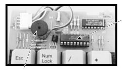
Carefully desolder and remove the original PIC from the board. Replace with the custom "Stamp Pad" PIC, using a socket if desired.
