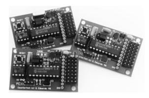
Figure 4. A trio of Stamp-compatible Counterfeit Controllers.
