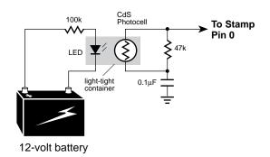
Figure 1. Battery-monitor setup.
