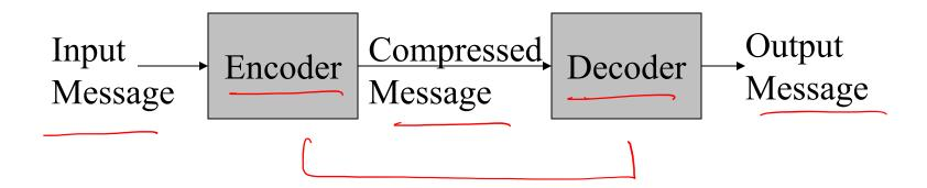
The encoder and decoder need to understand common compressed format.
