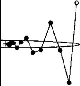
**FIGURE 6.3** Gradient descent on the simple quadratic surface of Fig. 5.10. Both trajectories are for 12 steps with  $\eta = 0.0476$ , the best value in the absence of momentum. On the left there is no momentum ( $\alpha = 0$ ), while  $\alpha = 0.5$  on the right.
