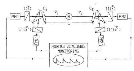
FIG. 2. Timing experiment with optical switches. Each switching device  $(C_{\rm I}, C_{\rm II})$  is followed by two polarizers in two different orientations. Each combination is equivalent to a polarizer switched fast between two orientations.
