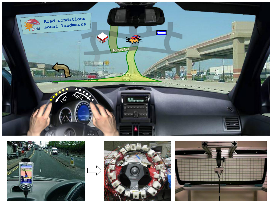
Fig. 2 Proposed sensory augmentation systems: Windshield-based AR navigation display ( top ) and haptically-enhanced steering wheel ( bottom center ) for providing vibro-tactile cues ( top )
