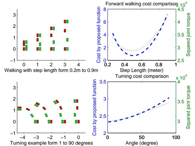
Fig. 4. Comparison between step costs by our simplified cost function and step costs by optimized humanoid walking motion. The blue line is the cost from Equation (10) and green line is the estimated cost from optimized human motion. Due to different scale size, the values are different between two cost results. However, they show a similar growth trend.
