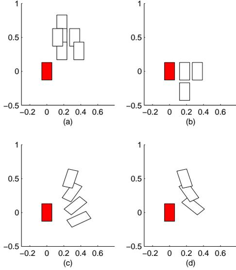
Fig. 5. Footstep action set with forward (a), sideways and backward (b), turn right (c) and turn left (d). The actions displayed are only those for the right foot (relative to the left foot shown in red).
