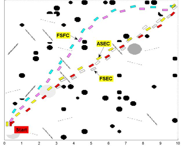
Fig. 7. Path planning in a large environment with size 10m x 10m; green and pink color step sequences is computed by FSFC with total step cost 16.9 and terrain cost 0.10; gray and white color step sequences is computed by FSEC with total step cost 12.3 and terrain cost 0.13; red and yellow color step sequences is computed by ASEC with total step cost 12.1 and terrain cost 0.23; the color map is an inverted gray scale color.
