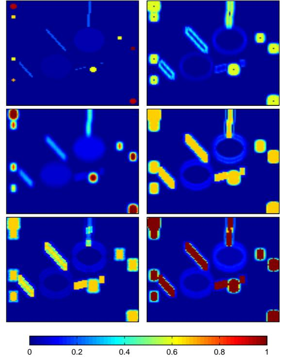
Fig. 1. Top left: terrain map with 4m x 4m size; Top right:  $C_{slope}$ ; Middle left:  $C_{altitude}$ ; Middle right:  $C_{rough}$ ; Bottom left:  $C_{bump}$ ; Bottom right:  $C_{Terrain}$ .
