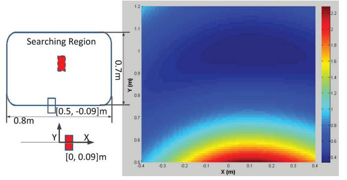
Fig. 2. Energy cost map per travel distance;  $l_p = 0.5$ ;  $SW = 0.178$ ; searching region in  $y$  direction  $[0.5, 1.2]$ m,  $x$  direction  $[-0.4, 0.4]$ m; the optimal step location is at  $[0.09, 1]$ m; the colormap is Jet in Matlab.
