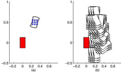
Fig. 6. Foot action with adaptive steps (a), adaptive steps with  $[-0.05, 0, 0.05]$ cm in x and y directions and  $[-\frac{1}{18}\pi, 0, \frac{1}{18}\pi]$  in orientation (b), overall coverage for 16 foot actions with adaptation.
