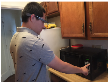
Figure 1: ApplianceReader is a wearable point-of-view camera-based system that combine crowdsourcing and computer vision to collaboratively label and recognize button controls on appliances, thus allowing visually impaired users to interactively explore and use appliances.
