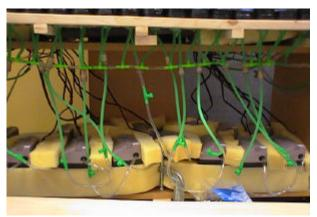
Figure 7. Sound Dampening Around Pumps
