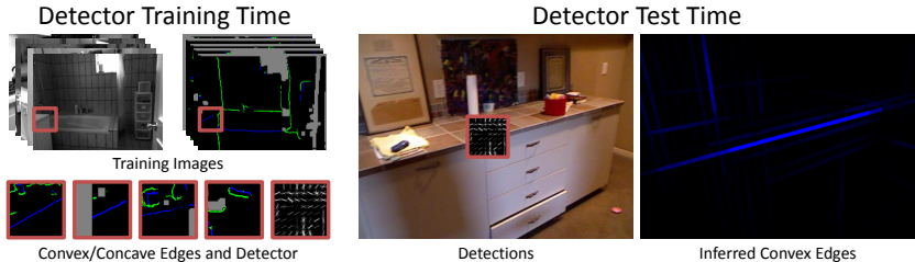
Fig. 5. An illustration of our approach for finding surface normal discontinuities. At training time, we automatically compute surface normal discontinuity maps (convex blue, concave green, missing data gray). At test time, we run a bank of 3D primitive detectors in the image; these detectors are trained to recognize a set of patches. We transfer the convex and concave edge patches associated with each detector.
