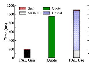
**Figure 2.** Breakdown of overheads that will be incurred by generic applications implemented in the SEA model. Measurements were taken using an HP dc5750 containing a 2.2 GHz AMD processor and a Broadcom TPM. PAL Gen represents the overhead for an application that generates data and seals it for later use. PAL Use unseals previous state, modifies it, and optionally reseals it.
