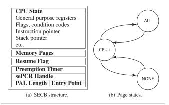
**Figure 5.** State machine for the possible states of a memory page in our proposed memory controller modification. The states correspond to which CPUs can access an individual memory page.
