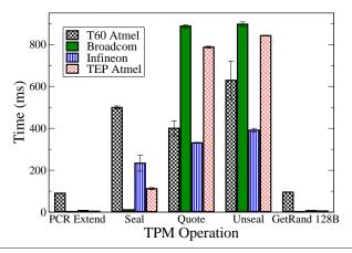
**Figure 3.** TPM benchmarks run against the Atmel v1.2 TPM in a Lenovo T60 laptop, the Broadcom v1.2 TPM in an HP dc5750, the Infineon v1.2 TPM in an AMD machine, and the Atmel v1.2 TPM (note that this is not the same as the Atmel TPM in the Lenovo T60 laptop) in the Intel TEP. Error bars indicate the standard deviation over 20 trials (not all error bars are visible).
