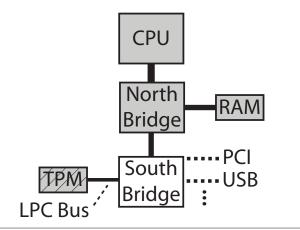
**Figure 1.** Chipset configuration for a modern x86 computer. Shaded components are part of the minimal TCB for our execution model. The TPM is shaded differently because it is included for practical reasons but is not an essential part of a stored-program computer architecture.
