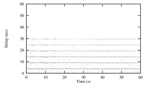
FIGURE 13. Packet delays vs. time, for a single RMTP/RTIP channel under non-real-time traffic congestion. The mean delay is 7.37 ms.
