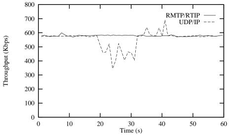
FIGURE 14. Throughputs of RMTP/RTIP and UDP/IP streams under non-real-time traffic load.
