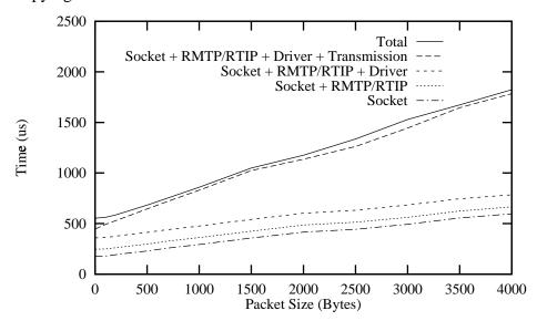
FIGURE 9. Breakdown of processing times in kernel for RMTP/RTIP send.
