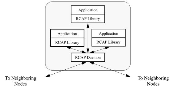
FIGURE 4. The RCAP library and daemon, within a single network node. Arrows represent RCAP control connections.
