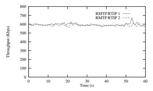
FIGURE 15. Throughputs of co-existing RMTP/RTIP channels under non-real-time traffic load. vic video sessions were run simultaneously from UC San Diego to UC Berkeley: one using UDP/IP from venezia to propaganda, the other using RMTP/RTIP from paola to faith. Both sessions had an average rate of 580 Kbps (roughly ten frames per second), a rate chosen to allow both sessions to get equal performance on an unloaded network.
