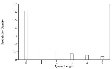
FIGURE 12. Probability density function of queue lengths, for a single RMTP/RTIP channel under nonreal-time traffic congestion. The mean queue length is 0.964.
