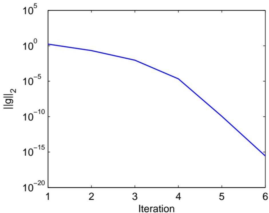
Progress of Newton's method on 3 bus example
