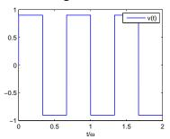
Can smooth through capacitors/inductors and also by switching more rapidly
