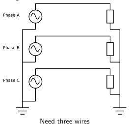
Attaching three wires in this manner known as a "wye" connection
