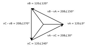
• Delta connector scales observed voltages by  $\sqrt{3}$
