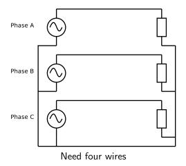
Because return wire has practically zero voltage, we can even eliminate it altogether
