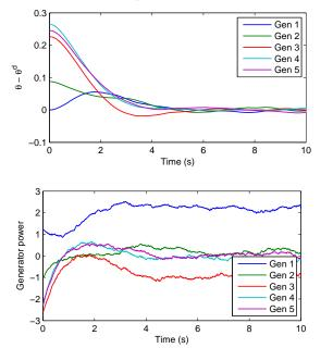
Can regulate generators more closely around desired point (at the expense of larger inputs)
