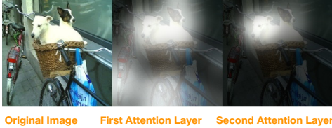
(b) Visualization of the learned multiple attention layers. The stacked attention network first focuses on all referred concepts, e.g., bicycle , basket and objects in the basket ( dogs ) in the first attention layer and then further narrows down the focus in the second layer and finds out the answer dog .
