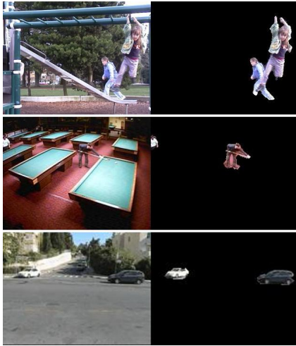
Figure 1: Segmentation results of typical frames. Each section is taken from a different sequence. The video of the girl shows a perfect segmentation result, the other two are lesser in accuracy but still good enough for most practice uses.
