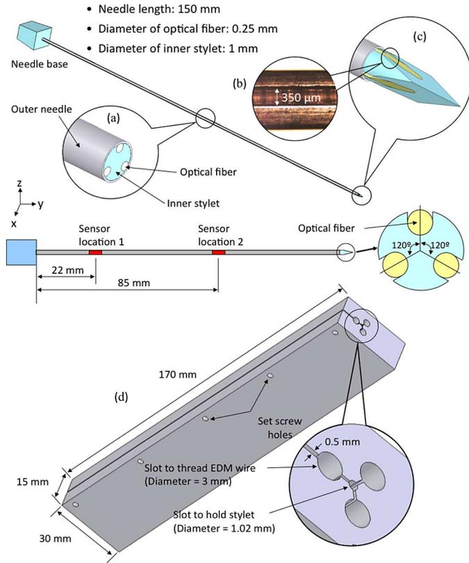
Fig. 2. Prototype design with modified inner stylet incorporated with three optical fibers. Three identical grooves at  $120^\circ$  intervals are made on the inner stylet to embed optical fibers with FBGs along the needle length. (a) Midpoint cross section. (b) Magnified view of an actual groove. (c) Tip of the stylet. (d) Fixture design for EDM parallel grooves in the biopsy needle stylet.
