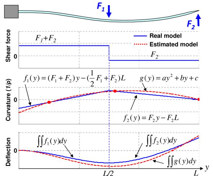
Fig. 1. Example of deflection estimation process based on beam theory. A needle is fixed at the base ( $y = 0$  mm), and two point loads of  $-0.6$  N and  $0.2$  N are applied at the midpoint ( $y = 75$  mm) and at the tip ( $y = 150$  mm) of the needle, respectively. The shaded dots in the curvature plot are sensor locations, which lead to an estimate for  $g(y)$ .
