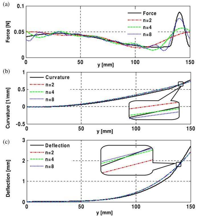
Fig. 3. (a) Force profile approximated with Fourier series with different numbers of terms. (b) Curvature profile—first integral of the force profile. (c) Deflection profile—second integral of curvature profile. The insets show the curvature and the deflection profiles are quite similar.
